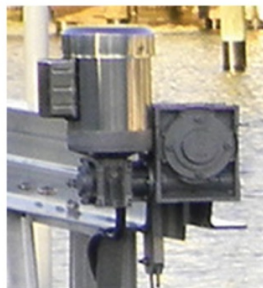
Synergy Gearbox and motor (Cover removed)
